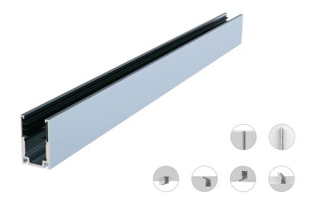
Specialized for the LED Flex Linear light, it was developed by combining the advantages of 6063 aluminum and elastic serrated tape. The inside elastic serrated tape as the grabbing force to keep continuous strong clamping force on the light body and protect the light from the damage caused by the large friction in the process of installation and dismantlement.
