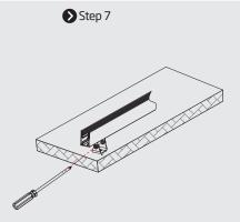
Tighten the side screws of pivot mounting bracket to avoid loosened locking point.
