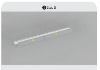
Cut one piece of inner aluminum profile evenly into two segments named 1 & 2 separately.
