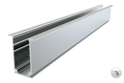
It uses high-quality 6063 aluminum with thin-wall, light- weight design to fit tightly the light body. It is deformation and rust resistant, and cost-effective. The "Flange" design is more suitable for recessed installation, better fits with the mounting groove and minimizes the operation tolerance during construction to some extent, like shielding the rough edges and the gaps of oversized groove.
